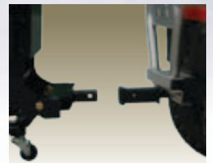
Drive Pro plows for utility vehicles attach using a 2" front receiver hitch mount
