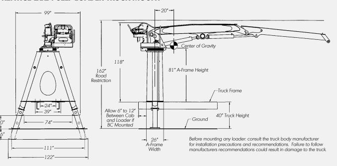
**Minimum Carrier** is a single axle truck with frame section modules of 18 cu. in. and GWW rating of 27,000 lbs. **Recommended Carrier** is a live tandem truck with frame section modules of 18 cu. in. and GWW rating of 32,000 lbs.
